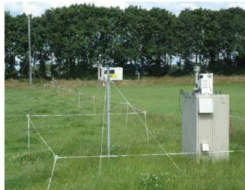
Measuring effects of a hedgerow on air quality along the Dutch highway A50 at Vaassen. Variability in the measurements is large and makes improvements hardly measurable.
