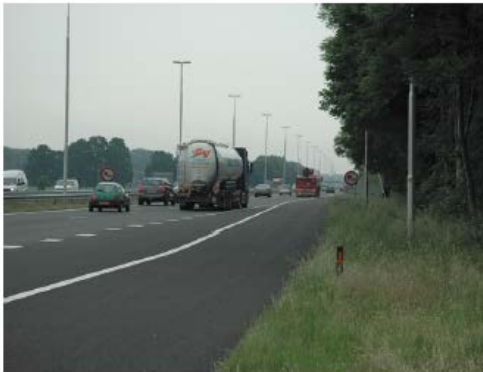
Measuring effects of a hedgerow on air quality along the Dutch highway A50 at Vaassen. Variability in the measurements is large and makes improvements hardly measurable.
